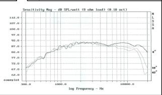
Measured on IEC baffle using Bruel & Kjaer 3144 model microphone.
